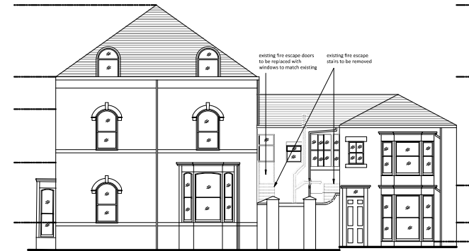
ELEVATION 03, RIGHT SIDE, LAWRENCE STREET SCALE 1:100
